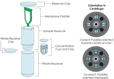
Figure 2: Buffer Exchange filter components and operation.
